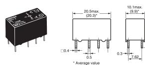
Note: Each value has a tolerance of ±0.3 mm.
